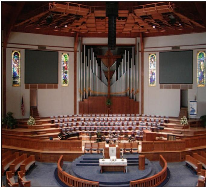
A central vertical line array design fits the architecture and room shape of Roswell First Methodist Church in Georgia. Pictured here is the JBL VerTec Series system designed by Brawley & Associates, with delay reinforcement from JBL AE Series and Control Contractor loudspeakers.
