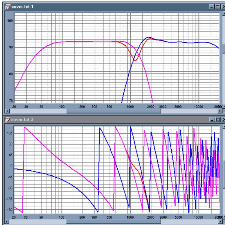
**Figure 9: Processing shown in Figure 6 with HPF and LPF replaced with 1.3kHz 24dB L.R. HPF and LPF. Pink – LF, Blue – HF, Red – Overall. Note the difference in phase response.**
