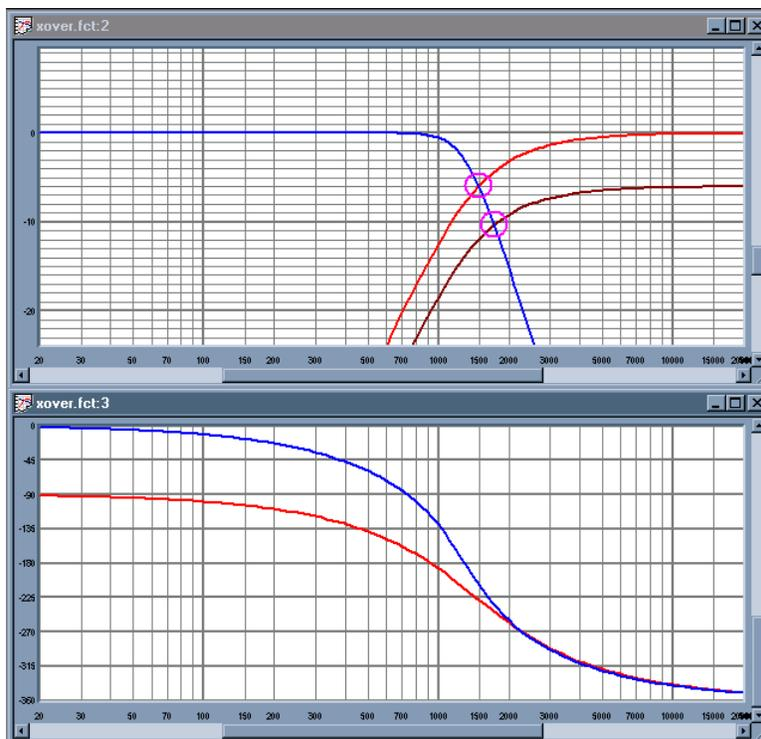
**Figure 13: Blue/Brown – LPF at 0dB, HPF at –6dB, crossover point at 1.7kHz. Blue/Red – LPF and HPF with +6dB gain change on HPF, crossover point now at 1.5kHz. Note that the red and brown phase responses overlap, so the brown phase plot is not visible.**
