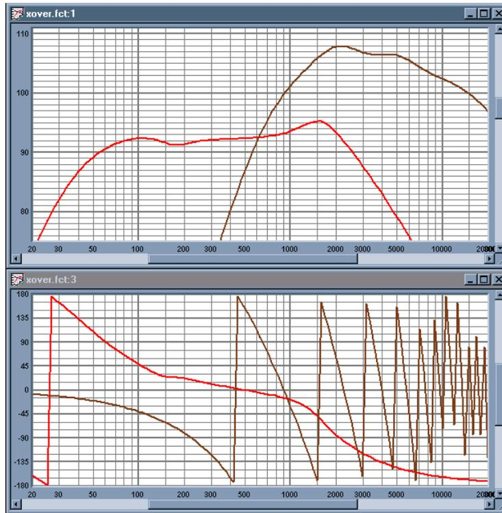
**Figure 5: Raw acoustical response of two transducers. Red- LF, Brown - HF. Crossover point at approximately 613Hz.**
