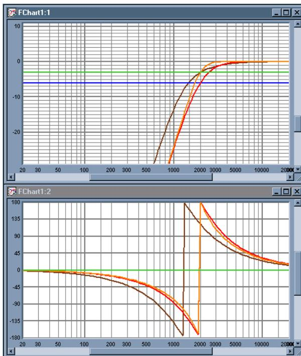
**Figure 1: Red- 2kHz 24dB Linkwitz-Riley high-pass filter, Orange – 2kHz 24dB Butterworth high-pass filter, Brown - 2kHz 24dB Bessel high-pass filter, Green – “-3dB”, Blue – “-6dB”**
