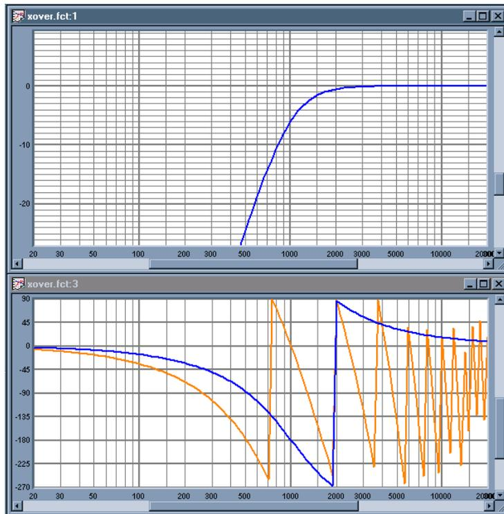
**Figure 3: Two identical filters. Orange - delayed, Blue - normal.**
