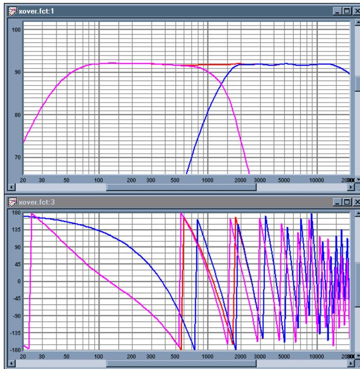
**Figure 7: Overall acoustical response of system with crossover. Pink – LF, Blue – HF, Red – Overall. Crossover point at approximately 1.3kHz**
