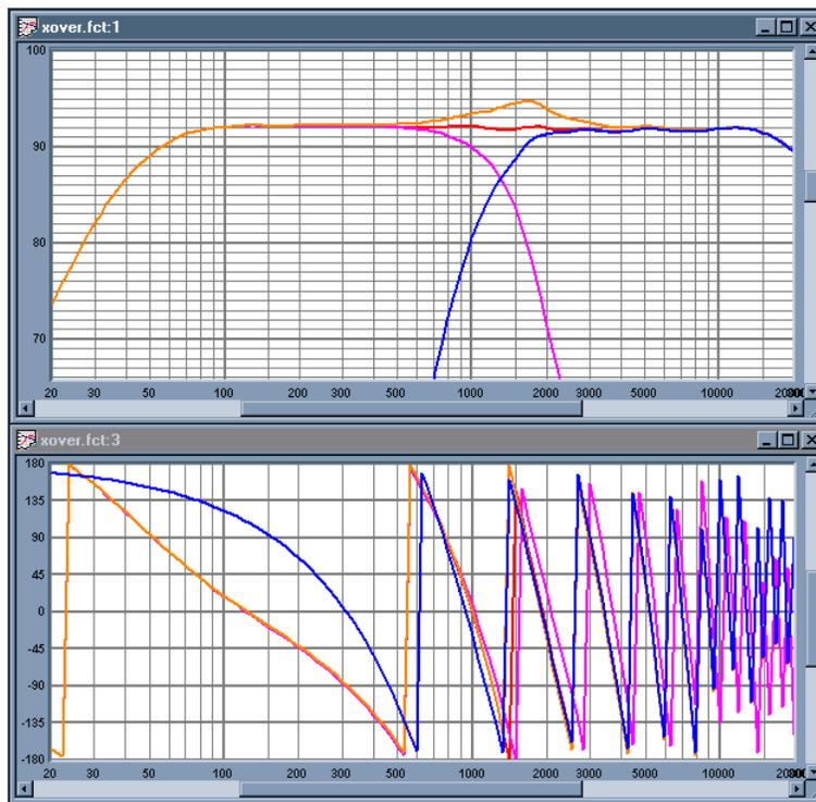
**Figure 12: Orange, system using 24dB symmetric L.R. filters with HF inverted. Red, final system with additional parametric EQ.**
