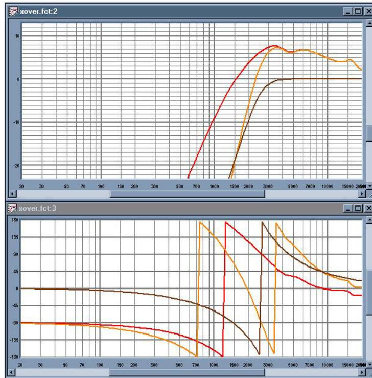
**Figure 4: Red – HF driver response, Brown – electronic high-pass filter, Orange - resultant response**
