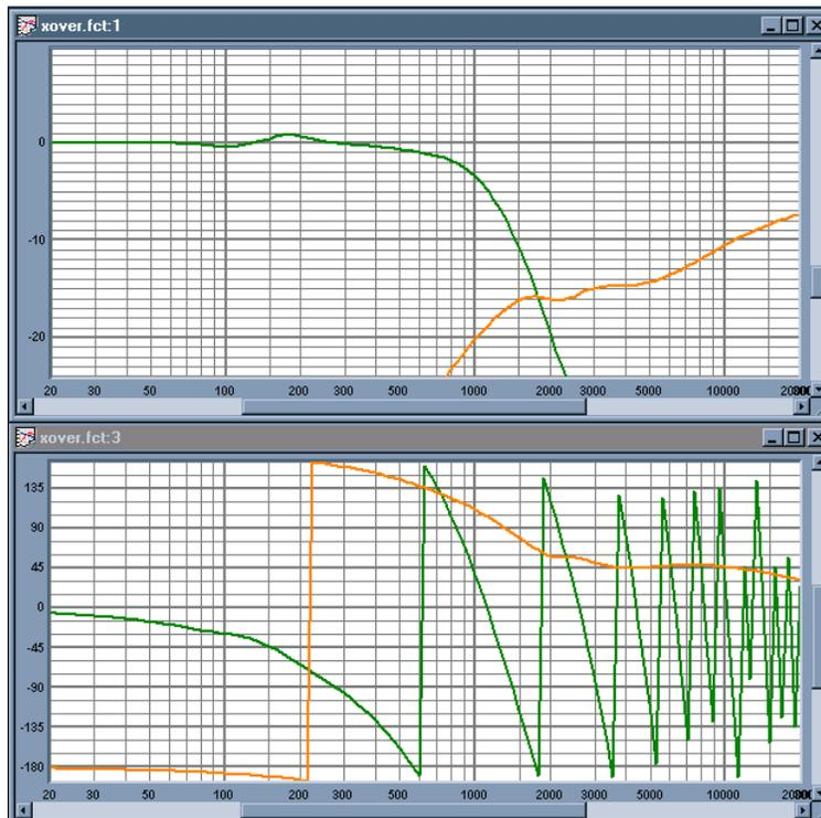
**Figure 6: Response of electronic crossover. Green – LF, Orange HF. Crossover point at approximately 1.8kHz**
