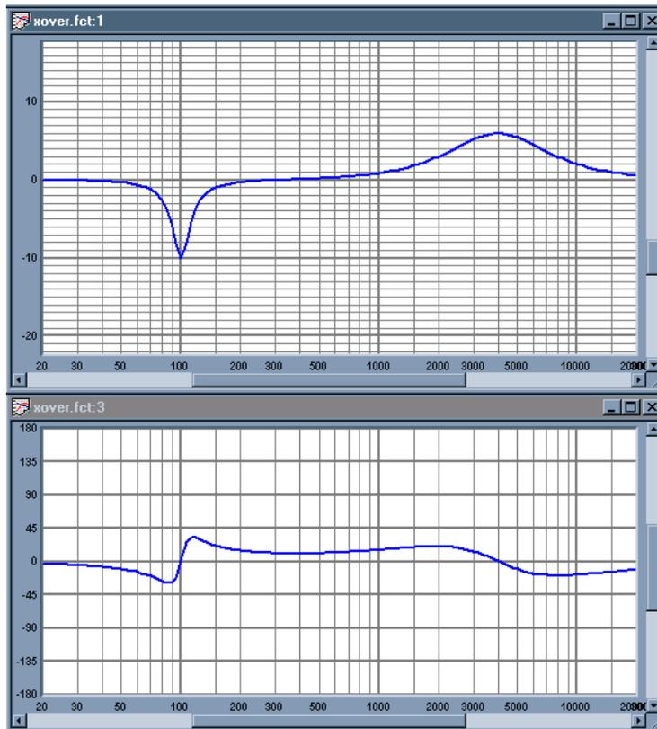
**Figure 14: Two parametric equalizers. 100Hz, gain of -10dB, Q of 6.3; 4kHz, gain of +6dB, Q of .67. Note the phase variations that accompany the magnitude changes.**
